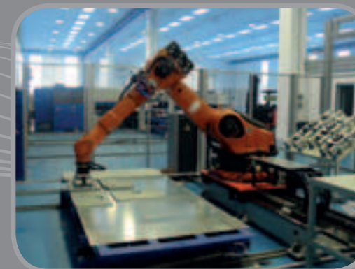
Carico e scarico pannellatrici Loading and unloading panelling machines
