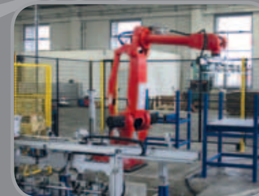
Scarico profilatrice Unloading profiling machines
