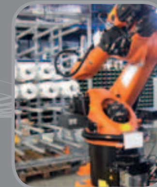
Carico e scarico bobine filato Loading and unloading yarn spools
